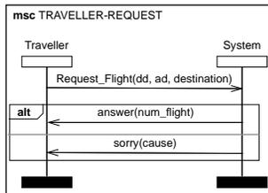
**Fig. 2.** MSC Traveller request use case diagram
