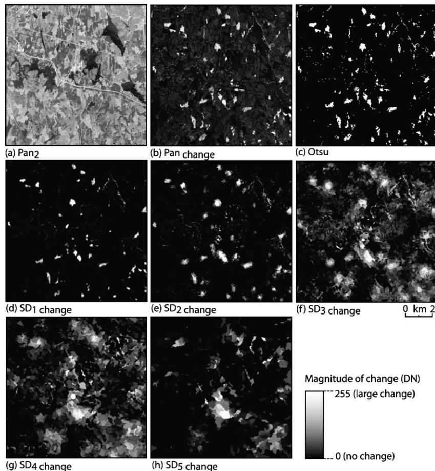
Fig. 5. Change dataset. Note that image (a) represents the original SPOT image, (b and c) represent the change dataset in original scale, and (d–h) represent the multiscale change dataset.
