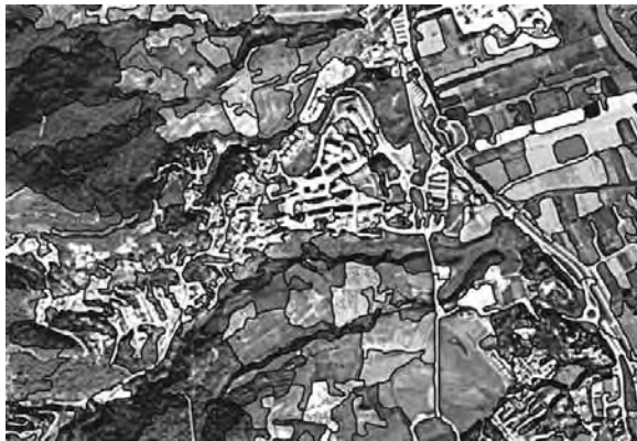
Figure 5. SCRM sample result in a SPOT5 multispectral (RGB 321) image (dimensions: 1.25 km \times 0.82 km). A color version of this figure is available at the ASPRS website: www.asprs.org .
