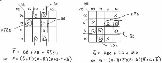
(c) [3 marks.] The K-maps below describe a system with three inputs and three outputs. Write equations for F, G, and H suitable for implementation on a PLA using the *smallest number of implicants*. Do not draw a PLA diagram.
