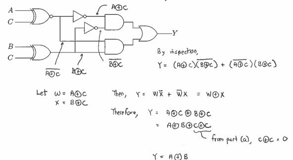
(c) [3 marks.] Use bubble-pushing and/or algebra to find a SOP expression for Y. If you use bubble-pushing, draw your equivalent circuit to the right of the given circuit. Hint for bubble-pushing with OR gates: A+B=
