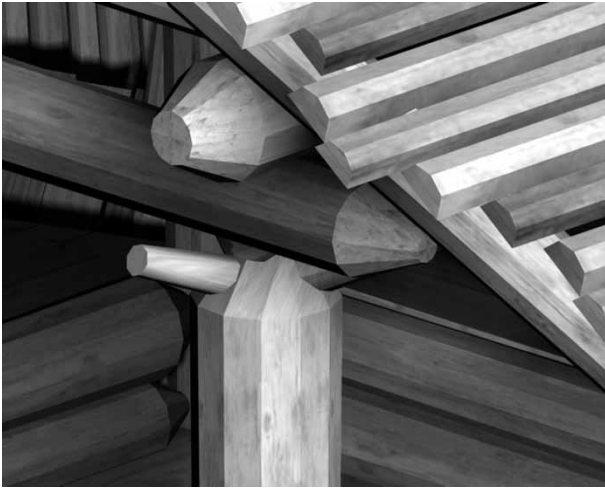
FIGURE 3. Post and beam construction, computer reconstruction.
