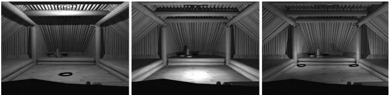
FIGURE 6. Lighting study. Right: single light source bottom centre. Middle: single light source from roof opening. Left: two light sources (lamps located on the left and right of the back sleeping platform).
