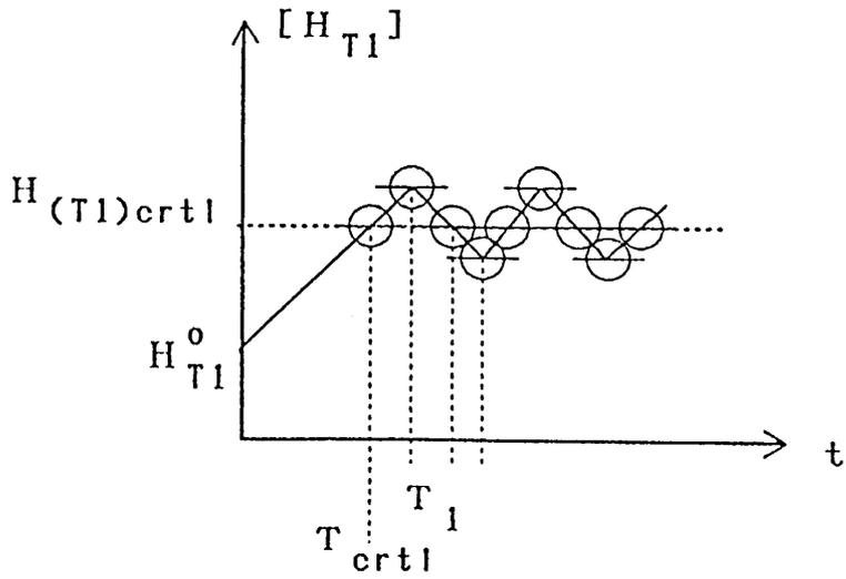
Fig. 9.3 Behavior for the tank  $T_1$  when the level passes a critical value
