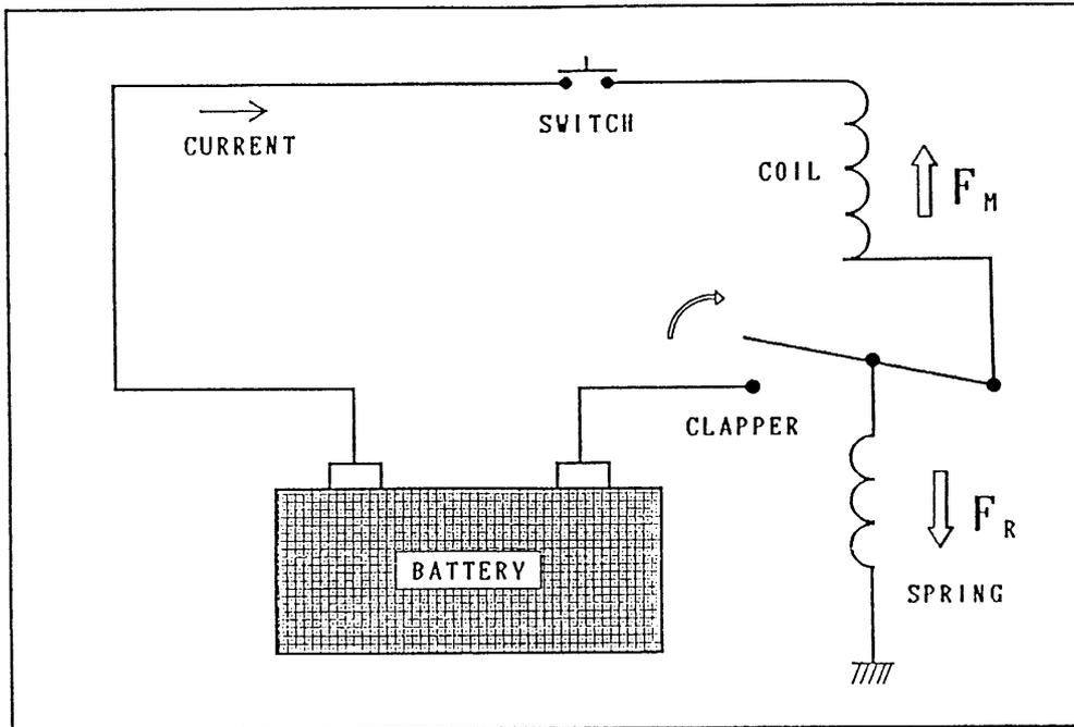
Fig. 10.5 Door buzzer
