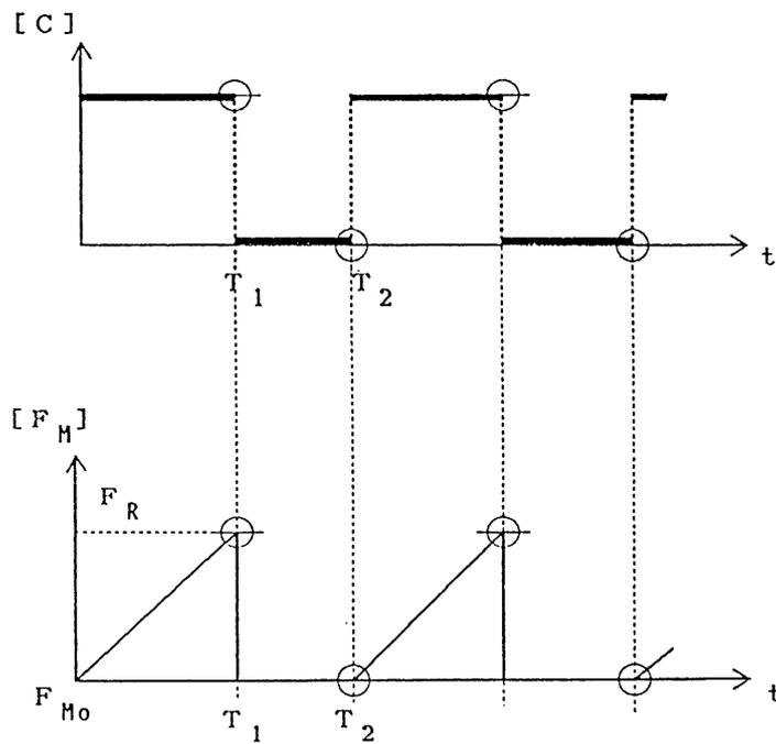
Fig. 10.6 Qualitative behavior of the door buzzer
