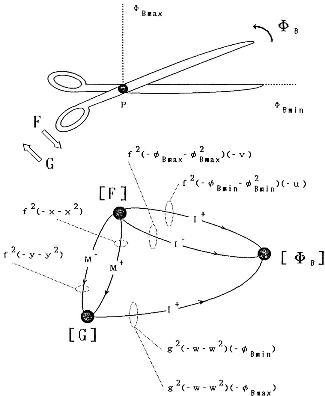
Fig. 10.1 TQFG for a pair of scissors
