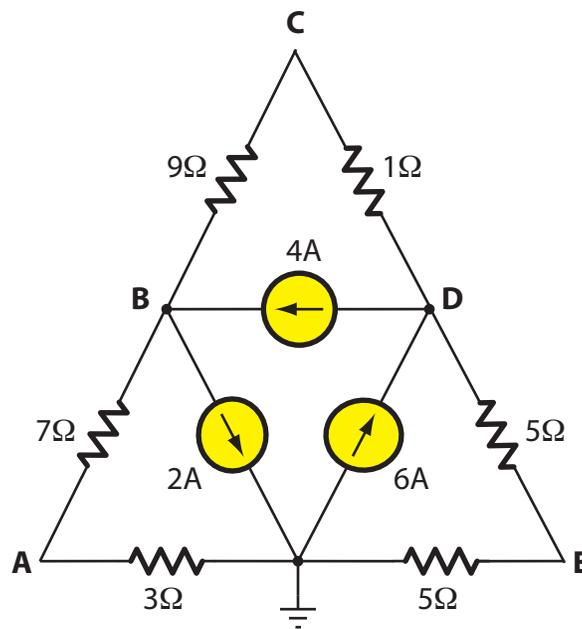
*Fig. P1. Find all node voltages and confirm energy balance*
