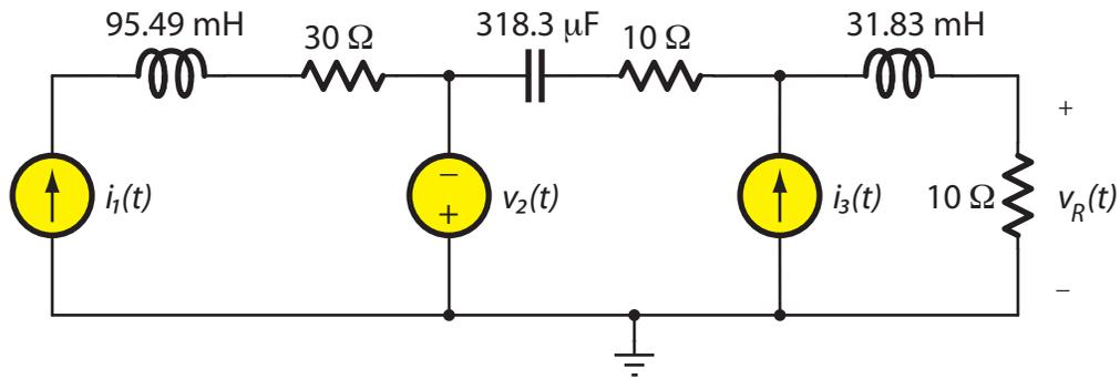
Fig. P2. Find  $v_R(t)$  by superposition
