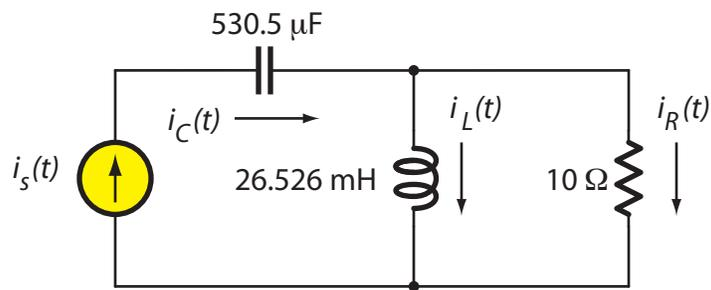
Fig. P2. Find  $i_C(t)$ ,  $i_L(t)$ , and  $i_R(t)$ , and average power in each circuit element
