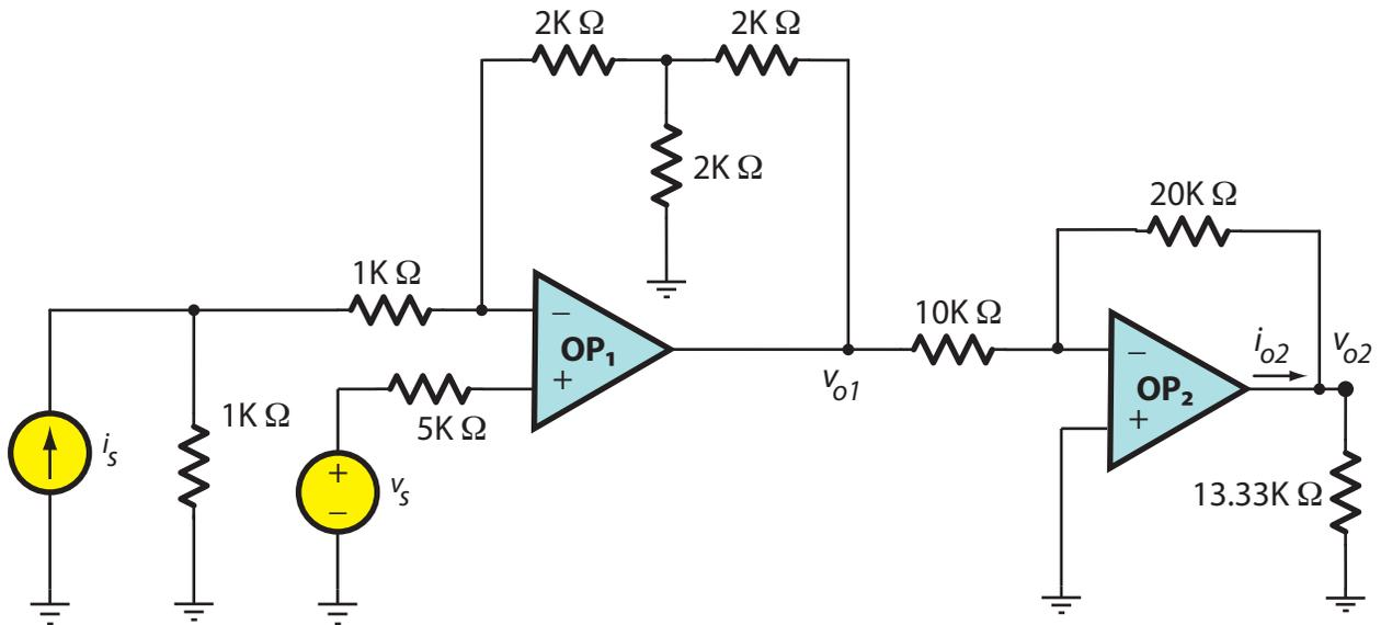
Fig. P4. Find  $v_{o2}(t)$ , output power of op amp OP<sub>2</sub>
