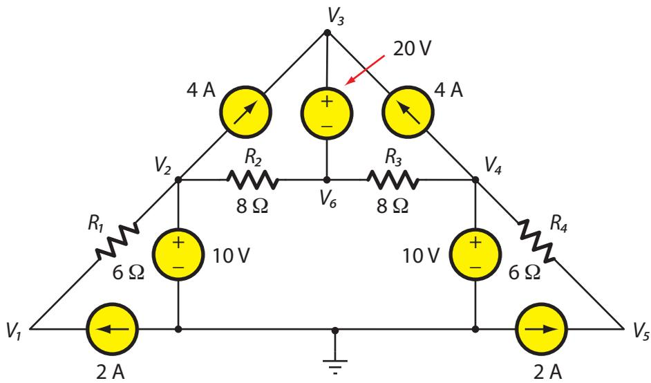
Fig. P1. Find the power in  $R_2$ , and find the node voltages
