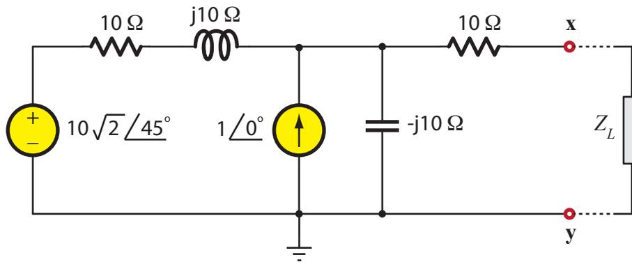
Fig. P4. Find the Thévenin and Norton equivalent circuits.
