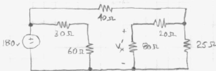
Note the 30Ω and 60Ω resistors do not influence  $V_x$  in any way
