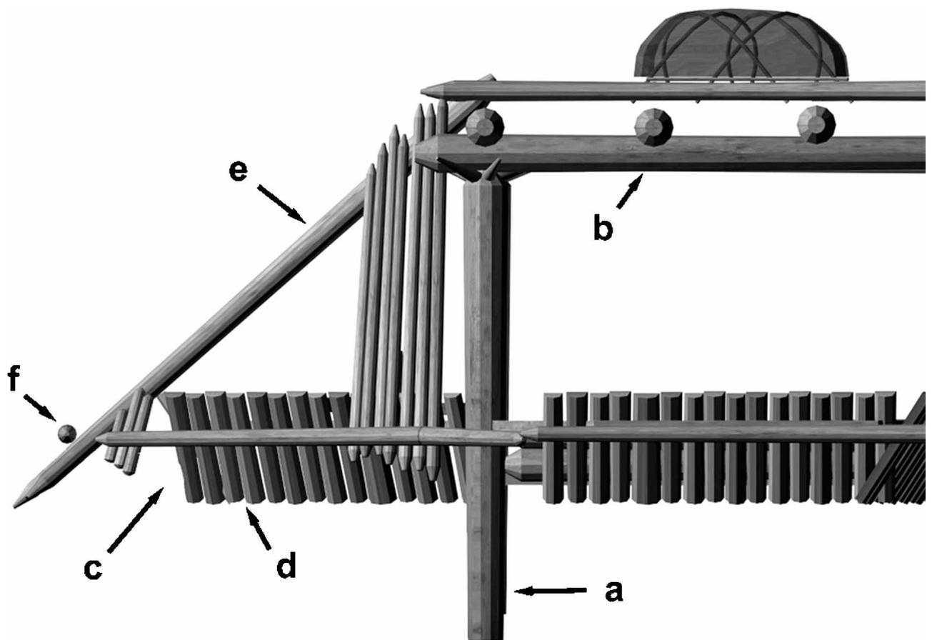
FIGURE 2. Section, final computer reconstruction: a, main supporting post; b, roof beam; c, pit; d, pony wall; e, log (abutment support); f, lean-to roof.
